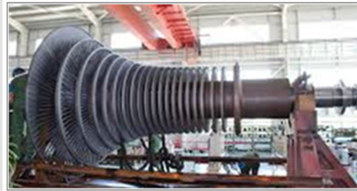
Figure 1: A conventional multistage steam-turbine rotor with progressively varying stage diameters.
