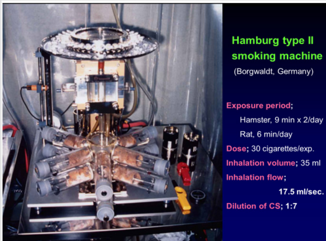
Figure 5: Ten Syrian golden hamsters exposed in the smoking machine and the different conditions of smoke generation between hamsters and rats.
