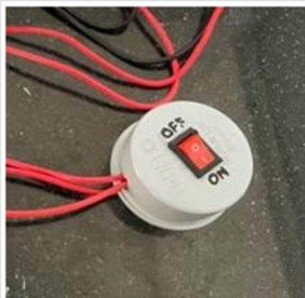
Figure 14: Polyvinyl chloride based ON/OFF switch with electrical wirings.
