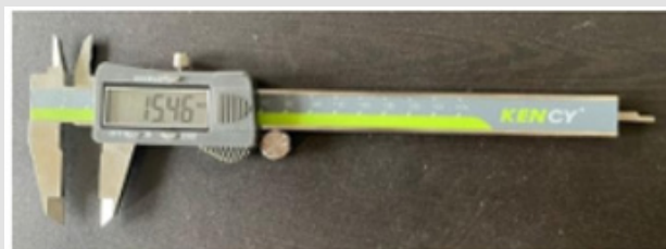
Figure 16: Digital vernier caliper to measure the dimensions of the flat container, measurement cup and bottle.
