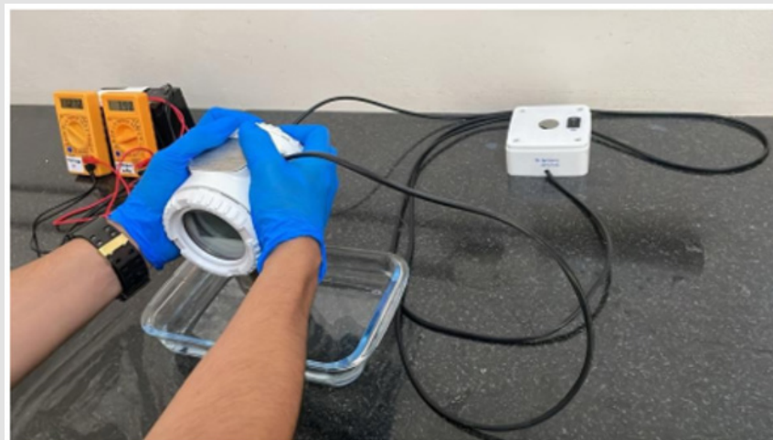
Figure 11: Pressure measurement of KCl inside the flat container. The pressure transmitter is connected to fluidic circuit. We perform experiments on 0.01 mol/litre KCl.
