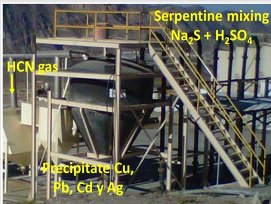
Figure 13: Simplified diagram showing the Serpentine process for copper, silver recovery and sodium cyanide recycle to the leaching circuit.
