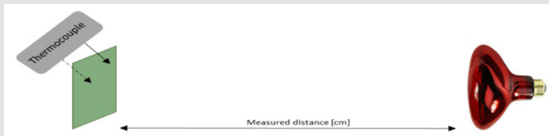
Figure 1: The experimental set up of IR lamp and PDLC film temperature measurement.
