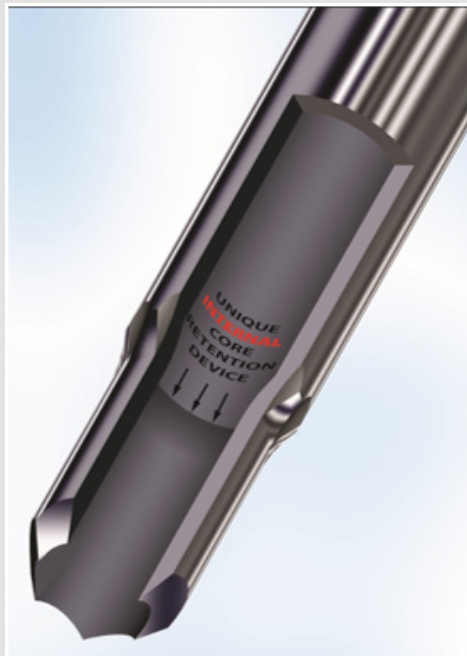
Figure 3: Cut section of the distal end of the needle showing the internal step and wider internal diameter.
