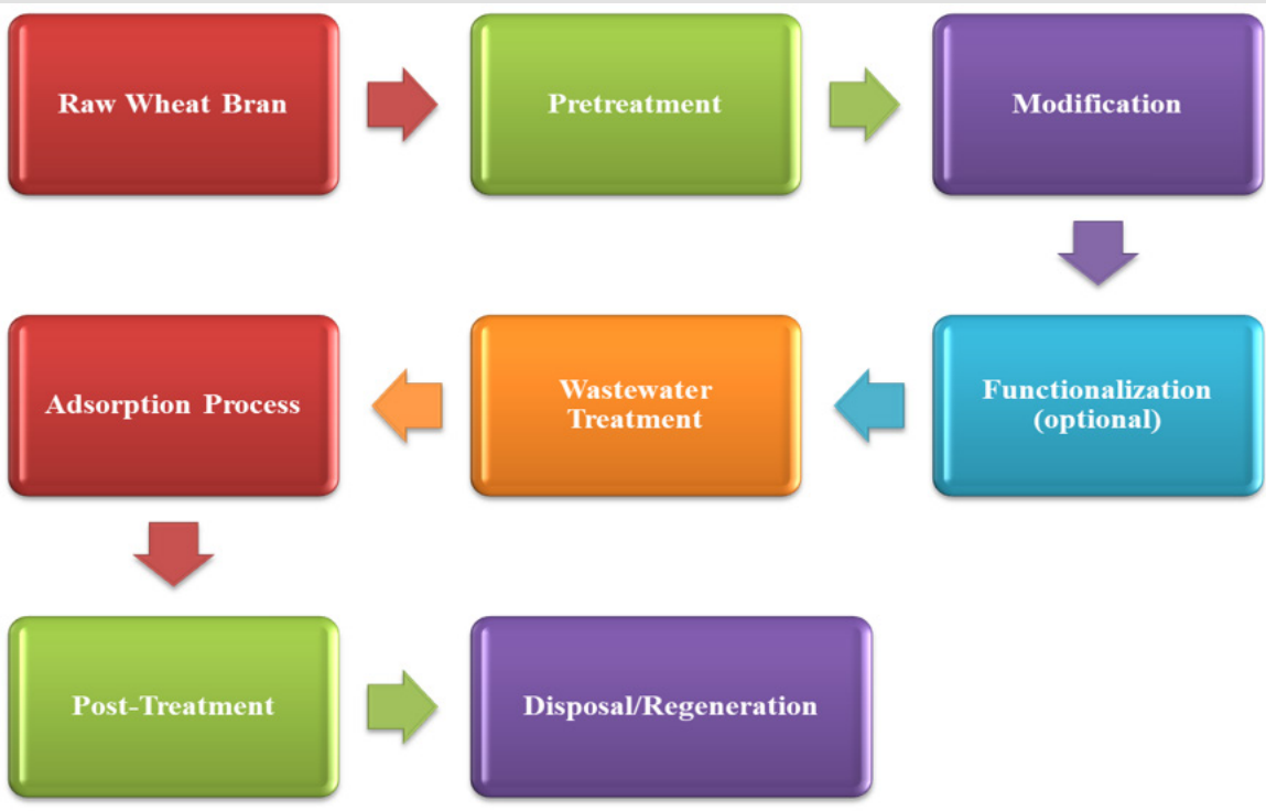
Figure 8: Schematic diagram modified wheat bran for the removal of heavy metals from wastewater involves specific steps to prepare the bran and then utilize it for adsorption.
