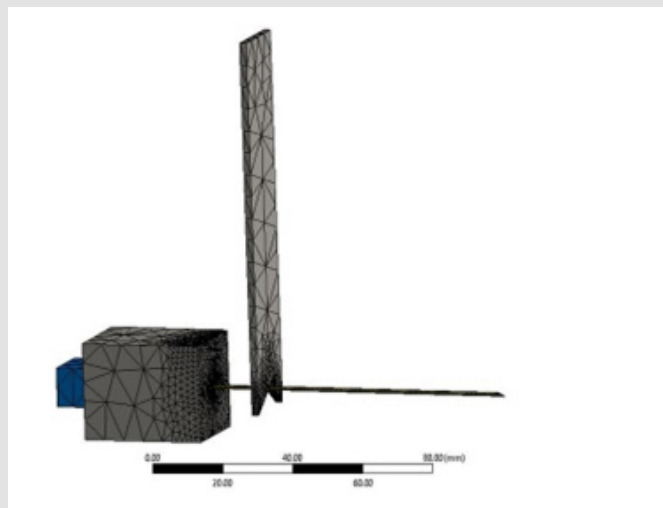
Figure 7: Meshing generation status for the bending setup and core needle.
