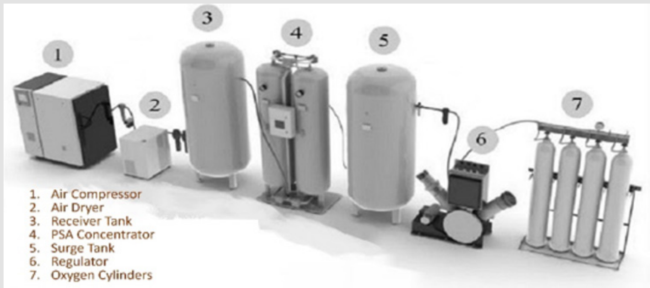
Figure 1: Process diagram of the PSA Medical Oxygen Production.
