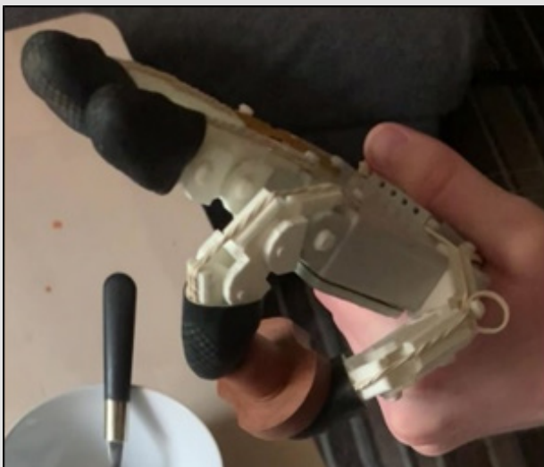
Figure 63: Prototype Thumb-index finger grasp.
