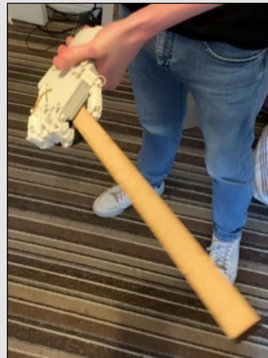
Figure 65: Prototype Medium Wrap Grasp.
