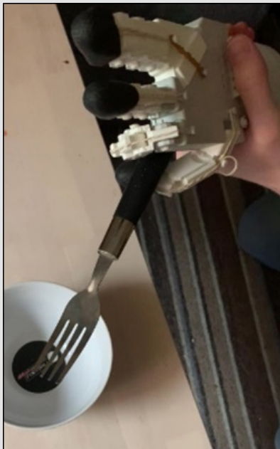
Figure 62: Prototype picking up fork (lateral pinch).
