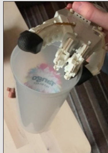
Figure 64: Prototype Thumb 2 finger grasp.
