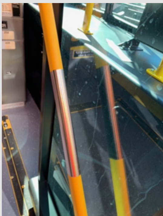
Figure 2: Antimicrobial copper on LA MTA bus entrance grab railing.
