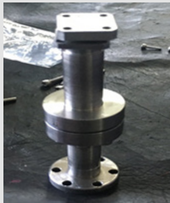
Figure 4: Photograph of the fabricated vacuum window.
