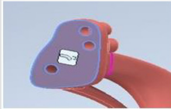
Figure 3: constraint on the top face.
