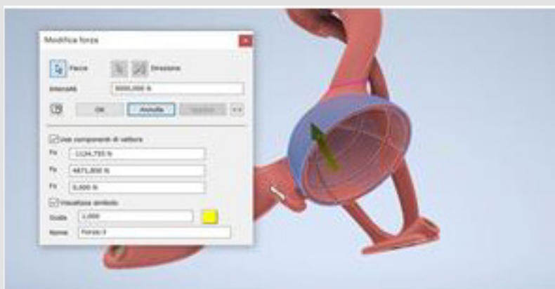
Figure 5: Load on the acetabular cup.
