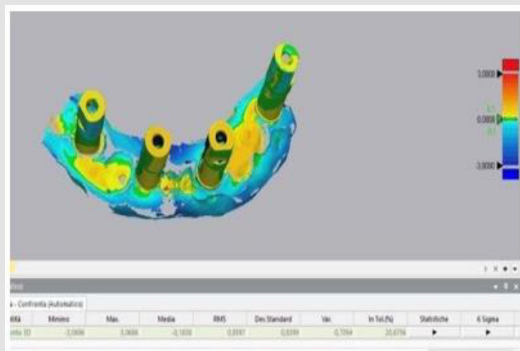
Figure 4: Comparison between stl control and stl with Commercial Scan Abutment.
