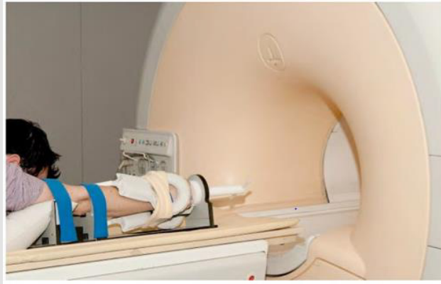
Figure 1: Jig prototype in use in an MRI machine with wrist coils attached.
