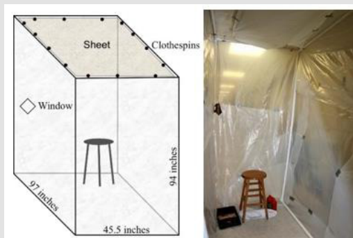
Figure 1: Room setup. The measurements of the room as well as the location of the supplies are shown. All the six sides of the structure were covered with the painter's plastic. A door was created with a flap of plastic for easy access. A window was also created opposite to the door for photo taking.
