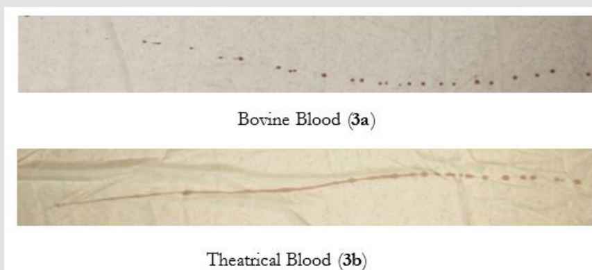
Figure 3: Representative Blood Spatter (7inch knife). Bovine blood a) Showed distinct, individual drops while theatrical blood. b) Formed a tail. Theatrical blood appeared to be less viscous and have less cohesive properties, making it more like water than like blood.
