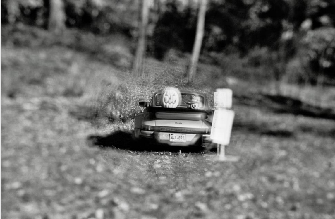
Figure 8: Figure 8 shows the model eye at F/11 with simulated LASIK ablation. The corresponding contrast sensitivity measurement is 4 and the central image quality is good.
