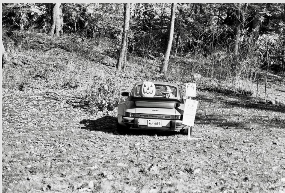
Figure1: Figure 1 is a photograph taken with the model eye at F/4 without simulated LASIK ablation. It has uniformly good resolution and contrast. The corresponding contrast sensitivity measurement is 4.
