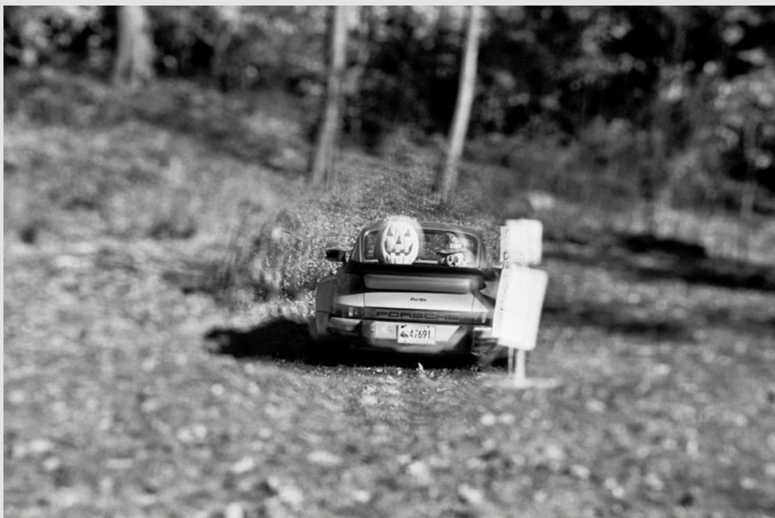
Figure 10: Figure 10 is a photograph with the model eye at F/16 with simulated LASIK ablation. The central image quality is very good, and the corresponding contrast sensitivity measurement is 4 .
