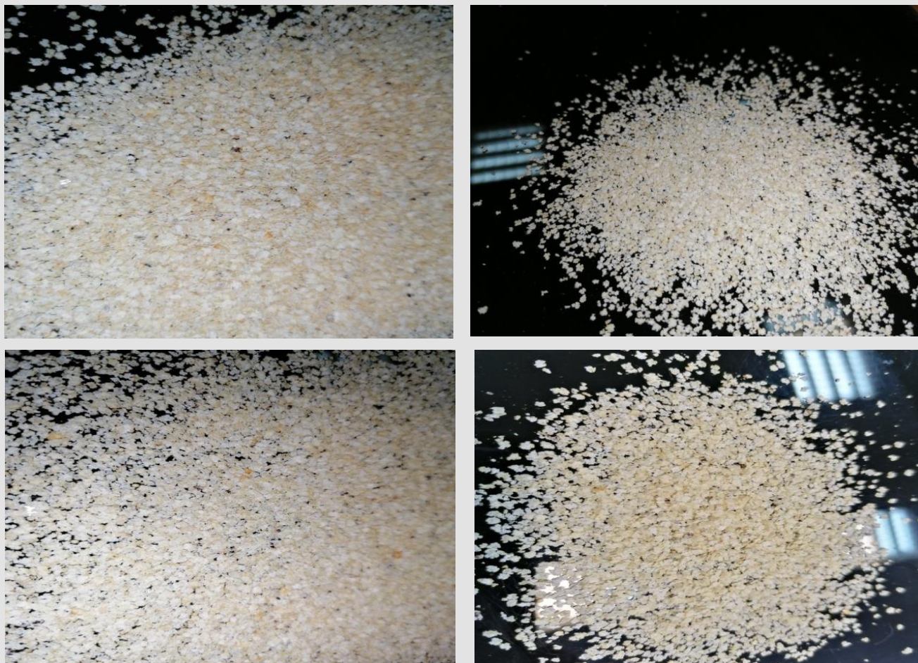
Figure 1: Appearance of amaranth flakes, depending on the size roller gap (a - gap = 0.3 mm, b - gap = 0.2 mm, c - gap = 0.15 mm, d - gap = 0.10 mm).
