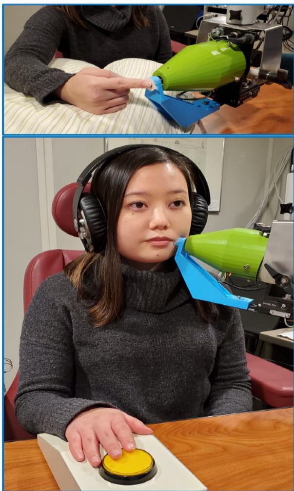
Figure 1: Test configuration for sampling vibrotactile detection thresholds at the glabrous index fingertip and oral angle.
