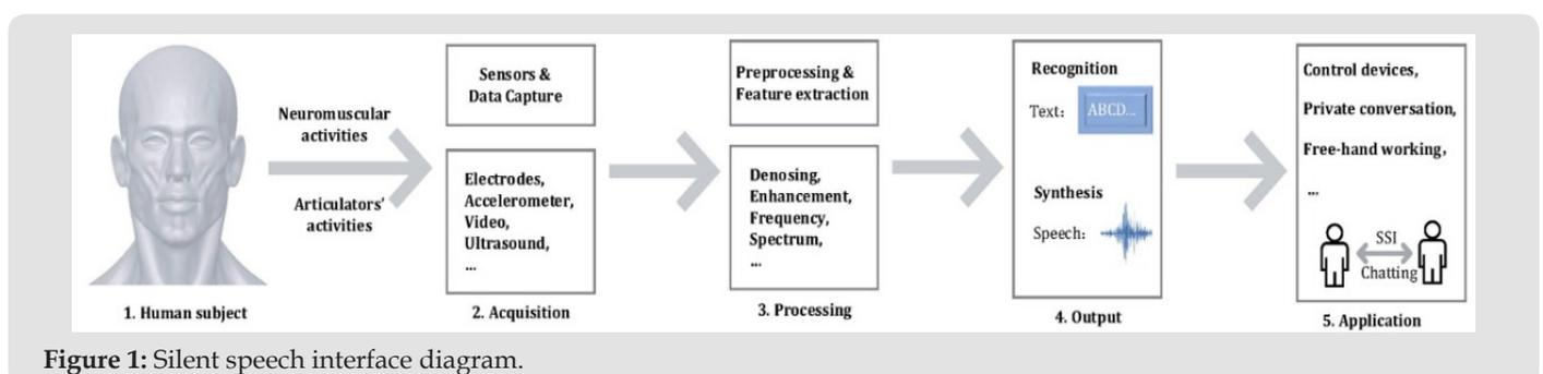
Figure 1: Silent speech interface diagram.
