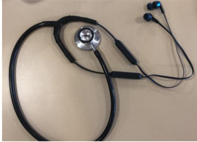
Figure 1: Hardware Simulator components: (Left) Stethoscope; (Right) Auscultation foci device.
