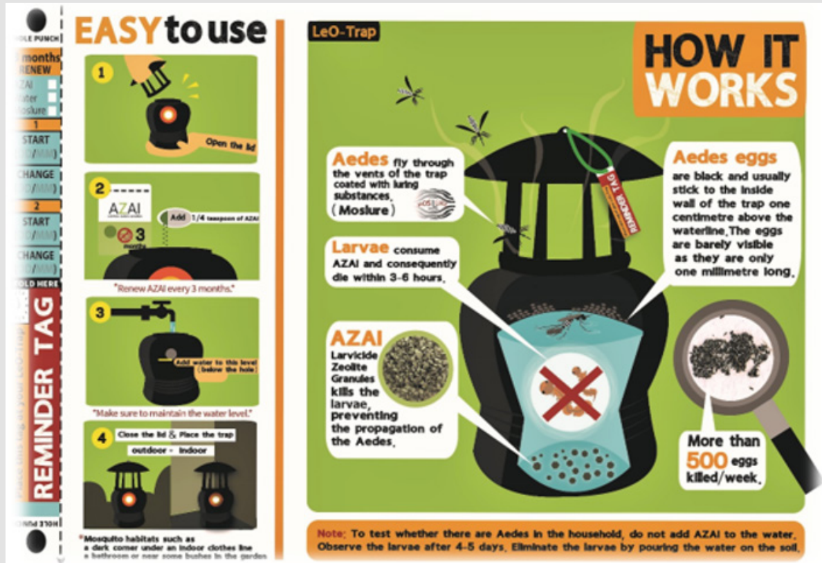
Figure 5: Instructions and explanations for users of the LeO-Trap® for controlling Aedes mosquitoes at home.
