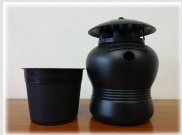
Figure 1: Comparison of the commonly used ovitrap (a black plastic cup) on the left and the newly developed ovitrap (LeO-Trap-V1) on the right.
