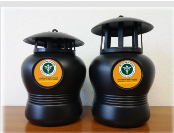
Figure 2: Comparison of the newly developed ovitrap (LeO-Trap-V1) on the left and the modified ovitrap (LeO-Trap-V2) on the right.
