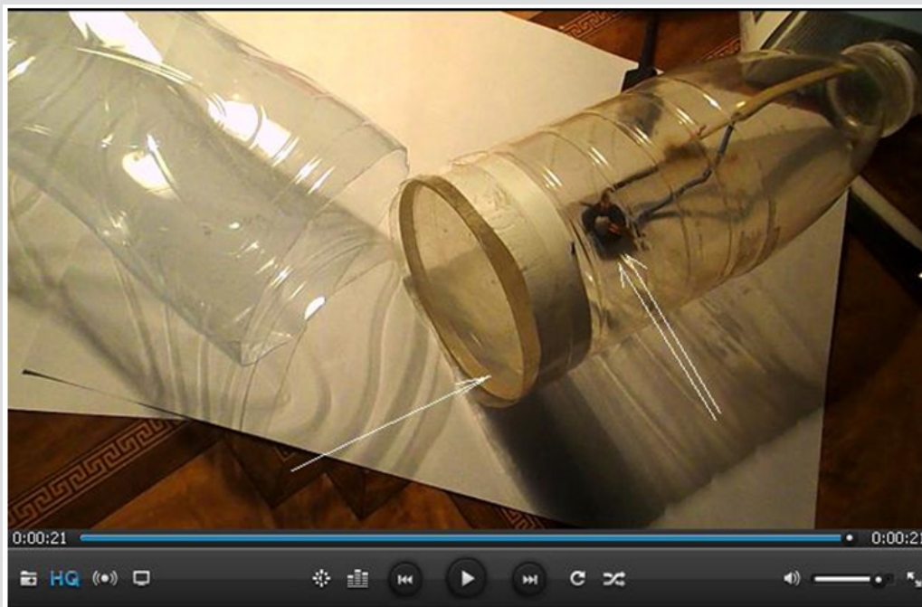
Figure 1: The photo of the initiating unit of the reactor. That unit contains CaF 2 window (marked by one white arrow) and the ferrite ring with two steel electrodes pressed to it (marked by two white arrows). The rest part of the reactor can be seen to the left from the initiating unit. Before the experiment it must be joined to the initiating unit at the CaF 2 end.
