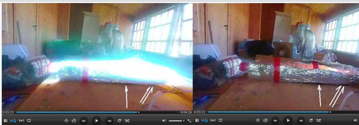
Figure 2: Two frames of video containing EEE in the reactor with CaF 2 barrier. The Air Inflammation filled the entire volume of the reactor in spite of barrier presence at the place marked by one white arrow. Two white arrows are showing at the place where the ferrite ring was positioned. The left frame contains the EEE image. The right frame contains the EEE afterglow image.
