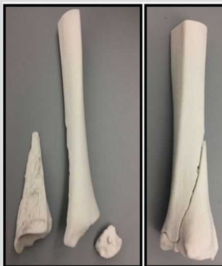
Figure 2: 3D printed model of a characteristic three-part triplane fracture, (A) Disassembled, and (B) Assembled. To print 3D fracture models, CT images of triplane ankle fractures were exported from Synapse (Fujifilm, Japan) into Mimics Medical software (Mimics, Belgium). 12 Fracture fragments were converted into a 3D mesh and exported to 3-Matic (Materialise, Belgium). The digital models were then transferred to Z-Print software and printed in a 1:1 ratio using a ZCorp 450 plaster powder printer (3DSystems, Rock Hill, South Carolina). Models were then coated with Permabond Adhesive 101 (Ellsworth Adhesives, Wisconsin).
