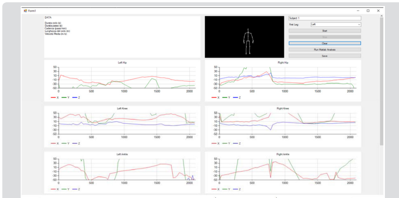
Figure 2: Kinect interface: measures of joints angles (hip, knee and ankle) along the three axes X,Y,Z.
