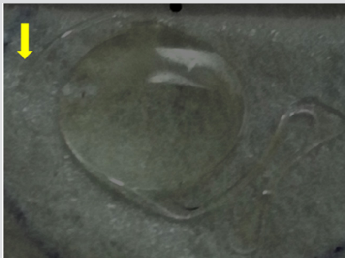
Figure 2: Photo of the intraocular lens fragments after explantation. Note that the fracture point is located at the proximal part of the lens loop.
