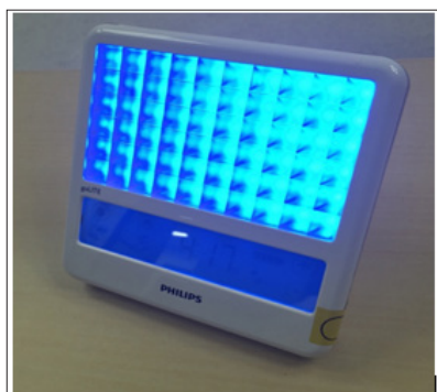
Figure 1: Philips goLITE BLU HF3331 for home use. The goLITE BLU is commercially available and has peak transmission at 470 nm, intensity at the cornea 300 lux, 2306 m-lux.
