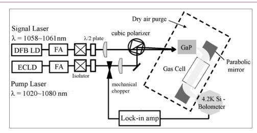
Figure 1: The optical setup for the THz spectroscopy measurement system for water vapor using LD pumped CW THz radiation.
