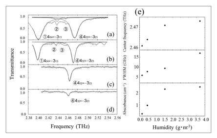
**Figure 3:** THz spectra of water vapor at different humidity levels at atmospheric pressure. The humidity is  $3.69 \text{ g/m}^3$  (a),  $1.55 \text{ g/m}^3$  (b),  $0.480 \text{ g/m}^3$  (c) and  $0.160 \text{ g/m}^3$  (d), respectively. (e) Dependences on humidity of the absorption peak position, the FWHM, and the intensity of the absorption band around 2.47 THz due to the rotational transition of  $4_{39} \leftarrow 4_{30}$ .
