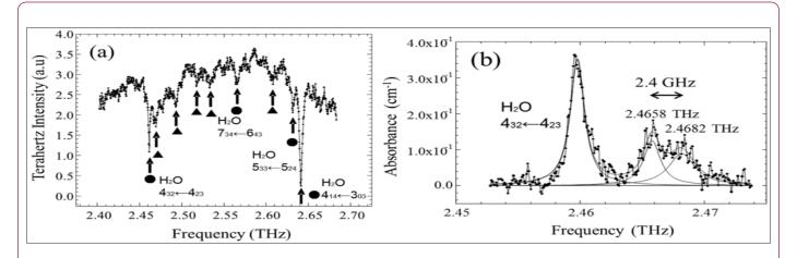
Figure 2: THz spectra of a mixture of saturated water vapor and ethanol at atmospheric pressure with frequency steps of  $3.36\times10^{-4}$  THz (a) and  $8.7\times10^{-5}$  THz (b), respectively.
