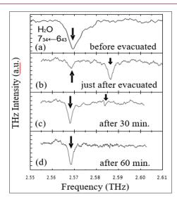
**Figure 4:** THz spectra of water vapor at a pressure of 14.6 kPa in a vapor-liquid coexistence: (a) before evacuation, (b) just after evacuation, (c) 30 min after evacuation and (d) 60 min after evacuation.
