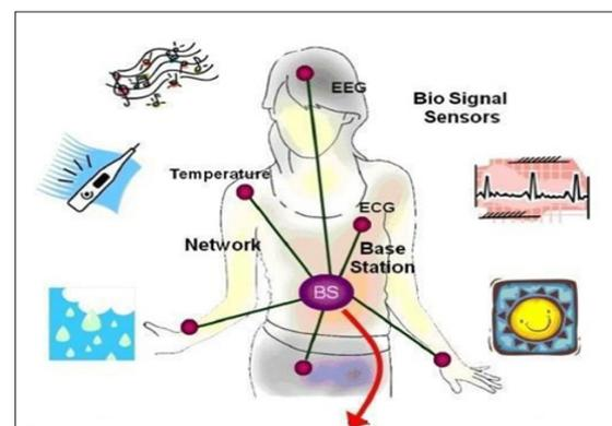
Figure 1: The Wireless Body Area Network.
