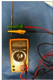
**Figure 2:** Measurement of the electrical resistance of a tapscrew.
