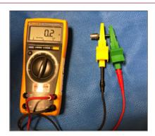
**Figure 1:** Measurement of the electrical resistance of a pedicle screw.
