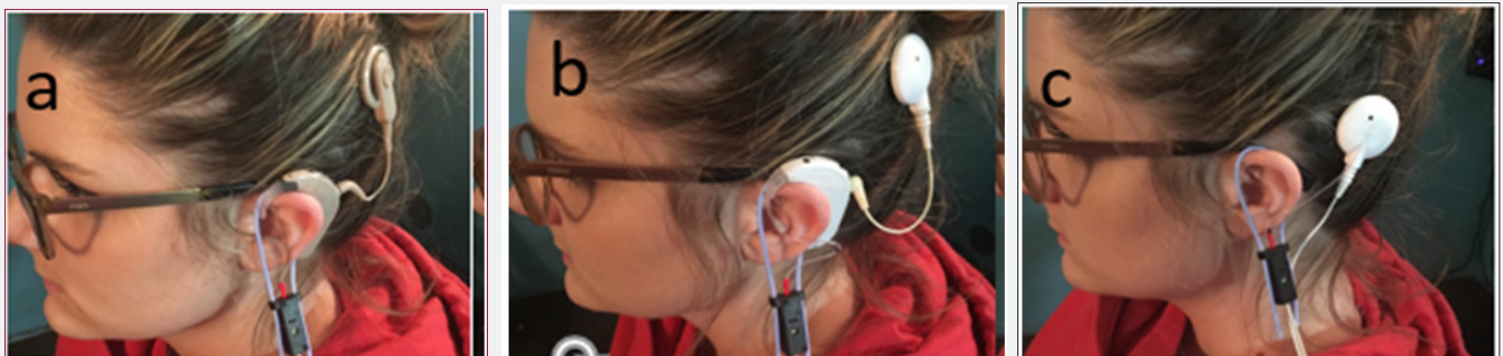
Figure 1: (a) The probe microphone is placed next to the processor microphone on the on-ear CI 1. (b) The probe microphone is placed next to the t-microphone on the on-ear CI 2 (c) The probe microphone is placed immediately below the microphone port on the headpiece of the head CI. The CI speech processor is not shown in the picture; however, it is clipped to the shoulder.
