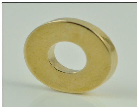
Figure 1: 3D printed investment casting for brass mold. Mold dimensions (5mm inner diameter x 2mm thickness).
