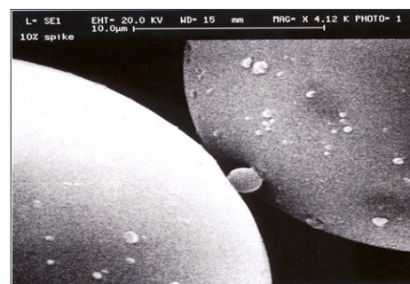
Figure 6: Small particles are attached to 40µm-microspheres. Small particles attached to 40µm PMMA.
