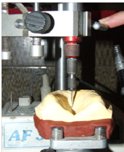
Figure 5: Pointed metal tip secured in the chuck of surveyor and positioned against the predetermined center on the master cast.
