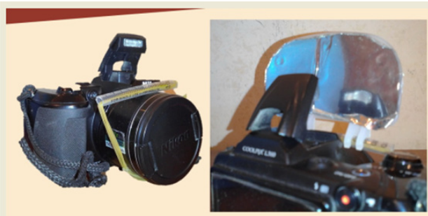
Figure 3: Customized flash reflector.
