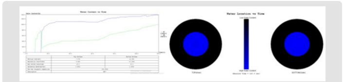
Figure 7: Water content vs. time (a) and water location vs. time (b) changes of fabric7.
