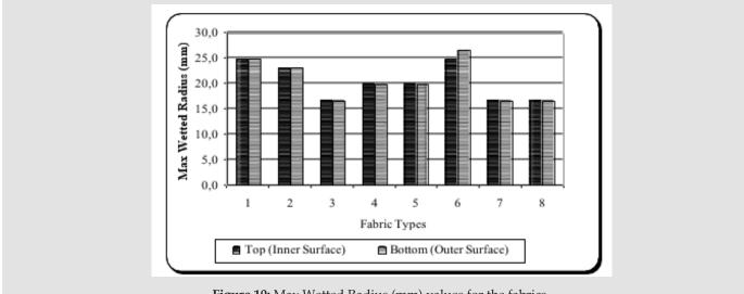
Figure 10: Max Wetted Radius (mm) values for the fabrics.
