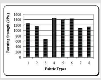
Figure 13: Bursting Strength values for the fabrics.
