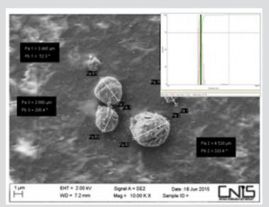
Figure 7: Chitin Nanofibrils-nanolignin biodegradable and smart carrier at SEM.
