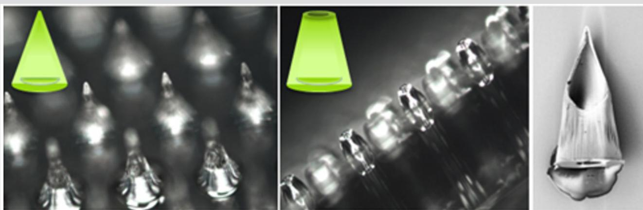
**Figure 1:** Schematics and images of polymeric MN: pyramidal shaped, conical shaped and hollow. Last image is highly detailed image of hollow MN realized by a scanning electron microscope.
