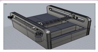
**Figure 2:** Thermal cycler mechanism with movement. Perspective of the complete machine. See, on the left part of thermal cycler, the pinion coupled to the tray in charge of the translation.
